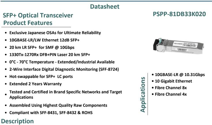
Platinum OEM Series PSPP-81DB33K020 is a Cisco Compatible Single Fiber BiDirectional 10GBASE-LR/LW Ethernet 10G Ethernet transceiver designed for long distance optical communications up to 20 km with signaling rates up to 10Gbps.
