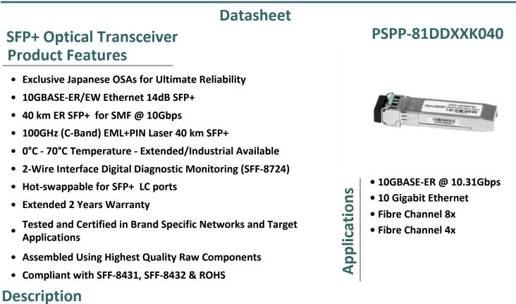
Platinum OEM Series PSPP-81DDXXK040 is a Cisco Compatible DWDM 10GBASE-ER/EW Ethernet 10G Ethernet / 8G FC SFP+ transceiver designed for long distance optical communications up to 40 km with signaling rates up to 10Gbps.
