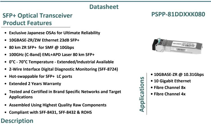
Platinum OEM Series PSPP-81DDXXK080 is a Cisco Compatible DWDM 10GBASE-ZR/ZW Ethernet 10G Ethernet / 8G FC SFP+ transceiver designed for long distance optical communications up to 80 km with signaling rates up to 10Gbps.
