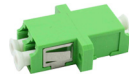
LC APC TO LC APC, SM DUPLEX ZIRCONIA CERAMIC SLEEVE SC FOOTPRINT P/N: OASS-KFDKFD-XXX
