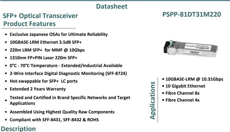
Platinum OEM Series PSPP-81DT31M220 is a Cisco Compatible Duplex 10GBASE-LRM Ethernet 10G Ethernet / 8G FC SFP+ transceiver designed for long distance optical communications up to 220m with signaling rates up to 10Gbps.
